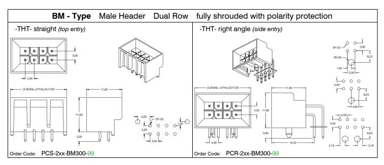
**Specification** Current rating 5 A Voltage rating 250 V AC max. Contact material Copper alloy 1000 M $\Omega$  min. Withstanding voltage 1500 V AC Insulator material LCP UL 94V-0 Insulation resistance Operating temp. -40°C to +105°C PCB thickness 1.60 mm Contact resistance  $10 \text{ m}\Omega \text{ max}.$
